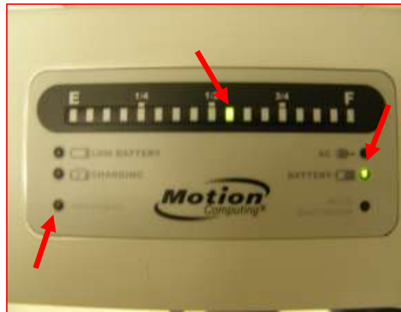
Figure 81. Checking the Battery Gauge
