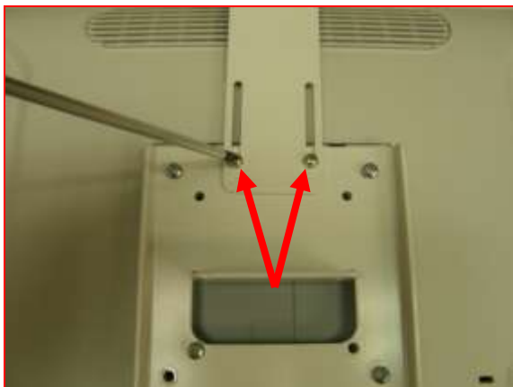
Figure 2. Screwing in Camera mount
