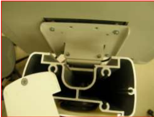
Figure 50. Placing Mount on the Bracket
