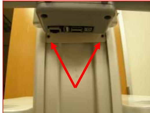
Figure 44. Securing the bottom 2 set screws
