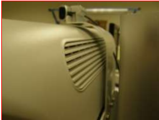
Figure 6. Placing Camera on mount
