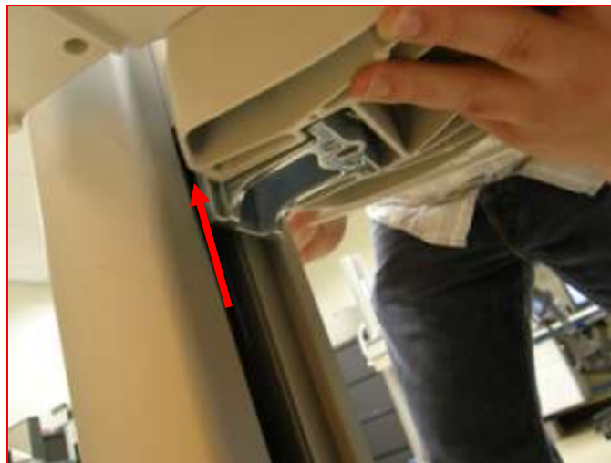
Figure 30. Sliding Large Work Surface up column
