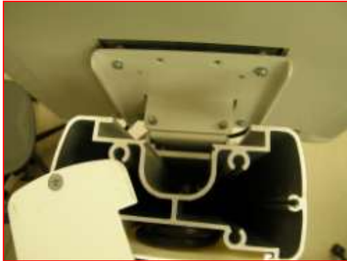
Figure 3. Placing the monitor on column
