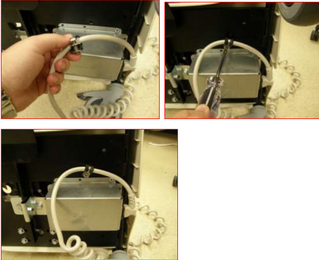
Figure 22. Attaching the Power Cord Retainer to the base
