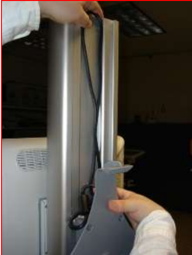
Figure 67. Looping VGA cable
