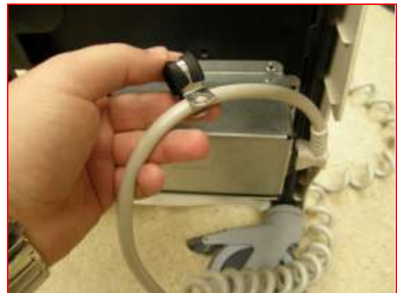
Figure 21. Put on Power Cord Retainer
