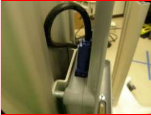
Figure 61. Tightening VGA cable
