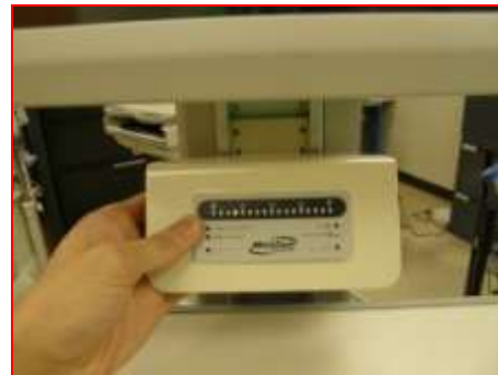
Figure 56. Placing Battery Gauge
