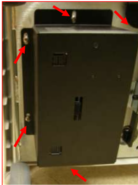
Figure 2. Showing where the screws are
