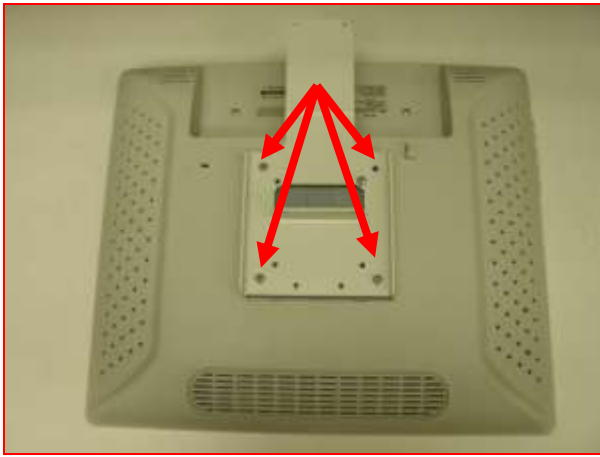
Figure 45. Screwing Mount to Monitor
