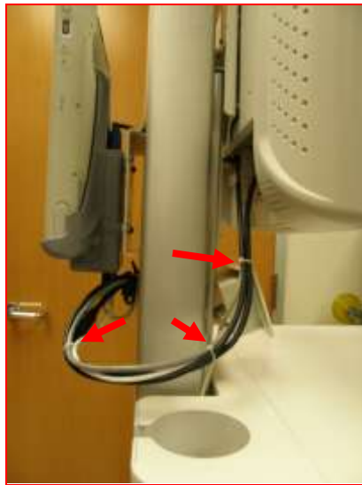
Figure 63. Securing with Cable ties
