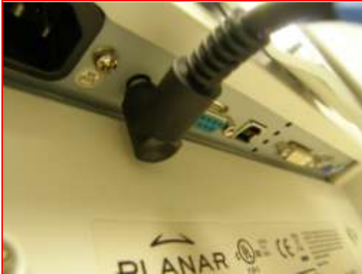
Figure 58. Plugging in Monitor Power cable
